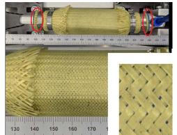
Fig. 1 Assembly of an untethered hydraulic actuated muscle.
