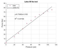
Fig. 2 Relation between force and pressure.
